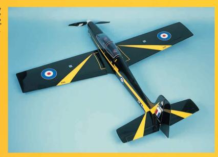
being the sizes of balsa involved. The 50% scale-up lends itself well to a  $^3/_8$ " wing,  $^3/_{16}$ " tail and  $^3/_{16}$ " fuselage sides, so the first job is to go and select the correct grades for the job. Try to use the softest, lightest sheets you can find (except where indicated on the plan) and you shouldn't go far wrong.
